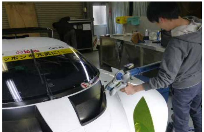
A Mooncraft employee demonstrates how the FARO Design ScanArm is used to scan components on a race car.
