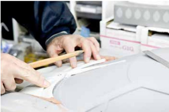
The process of attaching the 3D shaped part to the 1/5 model, to undergo wind tunnel testing. This helps Mooncraft to create a faster and safer car.
