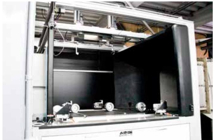
The wind tunnel test equipment used by Mooncraft.
